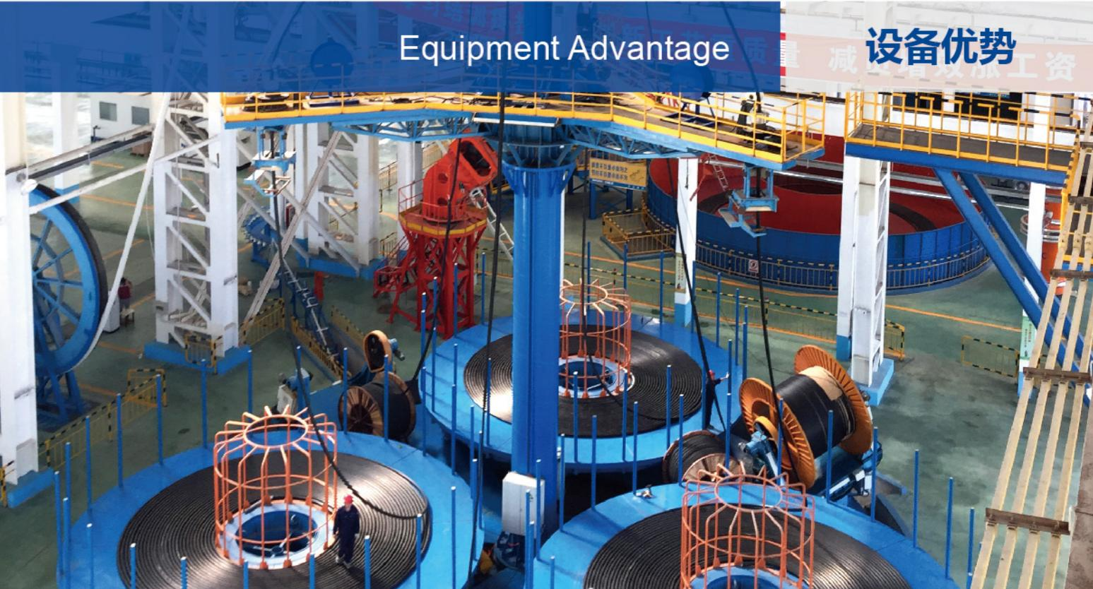
**Φ200+Φ120型挤塑生产线****Φ200+Φ120 type extruder manufacturing line**
